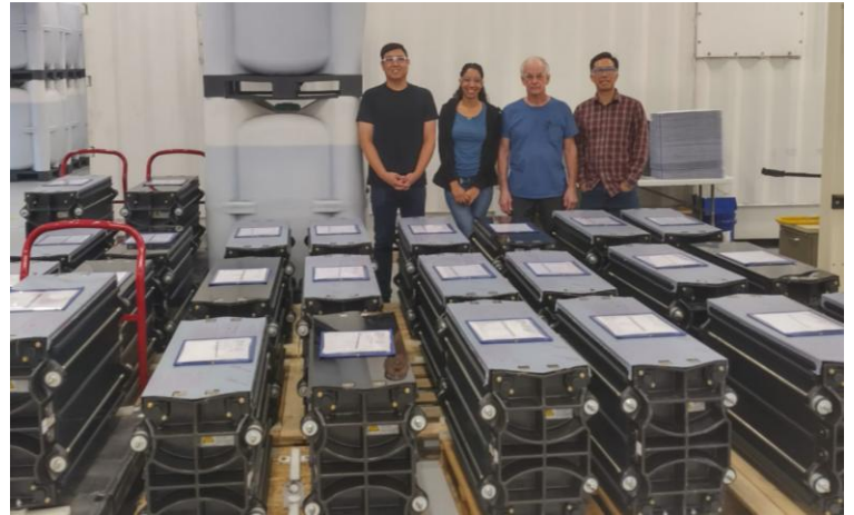
125-cell stack; \approx 40-kW with \approx 80% RTE
