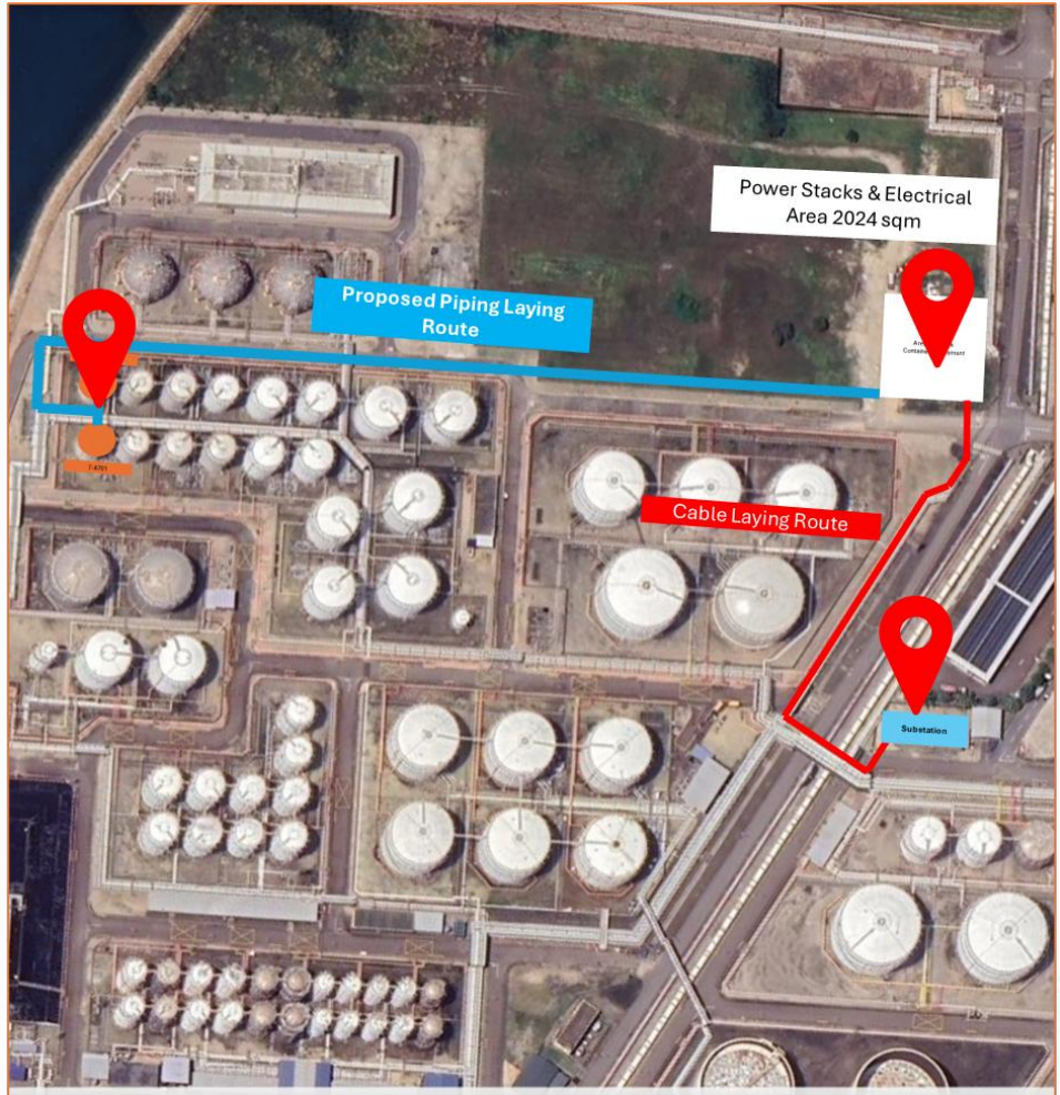
Piping Distance: ~400m, Cable Laying Distance: ~200m
