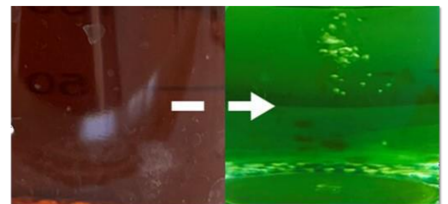
Figure 3: The image showcases the observable transformation in electrolyte coloration, indicative of the conversion from Fe 3+ to Fe 2+ .
