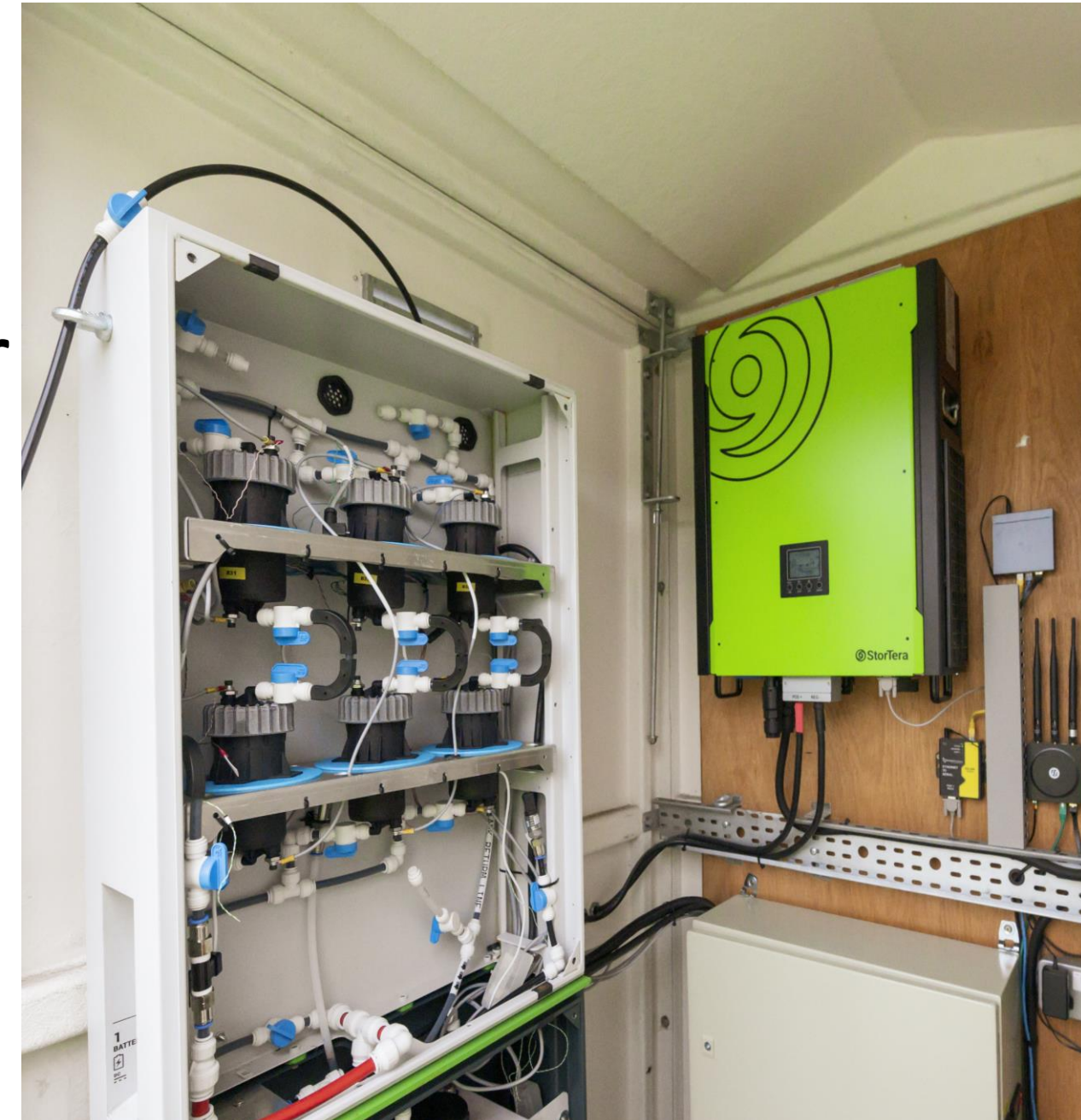
Figure 1: StorTera large scale lithium polysulphide test flow cell
