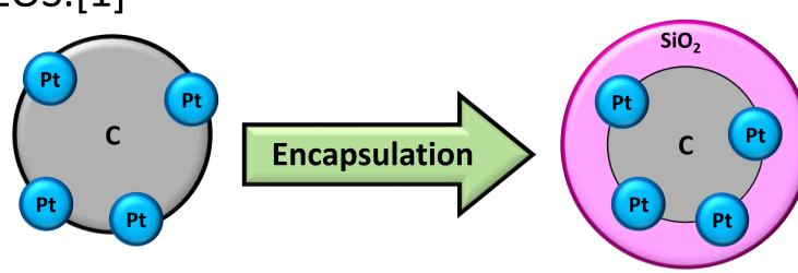
STEM-EDX confirmed the encapsulation of the Pt/C particles with a silica shell. Various Pt:Si ratios (i.e, overlayer thicknesses) were tested by accelerated degradation testing. The decline in electrochemically active surface area (ECSA) during prolonged potential cycling shows that the silica layer slows down catalyst degradation, increasing the half-life by a factor of 12 in 0.1 M HBr and by a factor of 4 in 2.0 M HBr.
