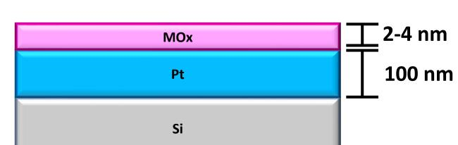
Electrochemistry combined with online ICP-MS was used to quantify the rate of Pt dissolution and study its potential dependence. SiO<sub>2</sub> and TiO<sub>2</sub> were found restore the typical platinum features seen commonly in weakly adsorbing electrolyte, suggesting that they successfully prevent Br from reaching the platinum surface whilst allowing for hydrogen transport.
