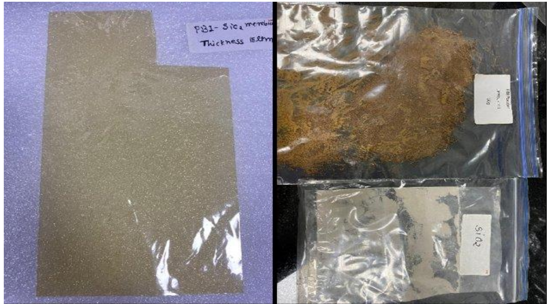
Fig. 1. Laboratory photographs of fabricated PBI–SiO 2 composite membrane samples. Left: cast membrane sheet (label indicates thickness 15 μm). Right: powder and fragment samples at different processing stages.
